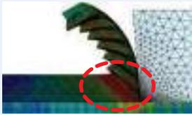
• Low heat conductivity in stainless steel machining involves high cutting heat and shear chips, all of which are **concentrated on the cutting edge**
